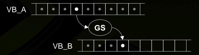
Geometry Shader allows variable output A single emitter particle spawns many output particles
